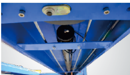
▲ High quality hydraulic cylinder utilizes imported oil seals.
